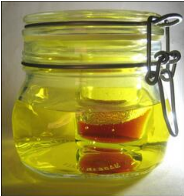
17oct'21 500ml container with 250ml water. "shot glass" with 5g SCF+5.5ml water plus 5g CAC+4.5ml water. Photo at +30 minutes.
